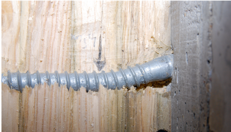
Figure A1-8 : Plastification du tirefond
