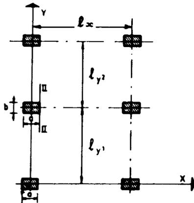
$$V_{ou}^{II} = V_u^{II} \frac{\frac{l_{y1} + l_{y2}}{2} + b}{l_{y1} + l_{y2}}$$
